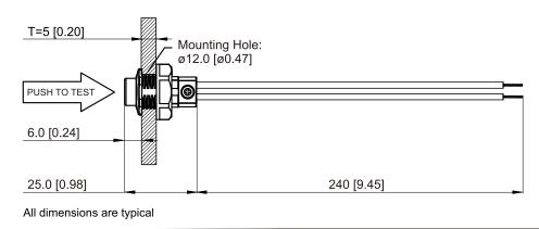
Dimension unit: mm [inch] Tolerance: ±1 [0.04]
